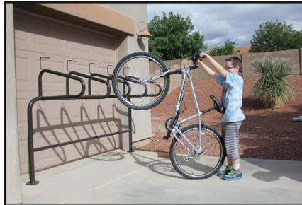
Pull Back on Handlebars using seat for leverage
