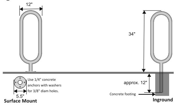
Dimensions are reference only. Stainless version dimensions vary slightly. Use actual units for core hole dimensions
